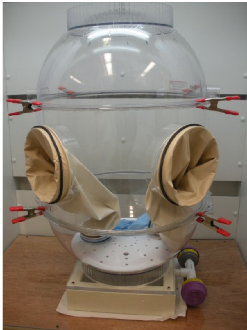
Figure 5. Secador® Techni-dome® 360 Vacuum Desiccator with 30-cm (12-in) extension ring outfitted with glove ports. Note the spring-loaded hand clamps used to keep the environmental test chamber tightly sealed. (Photo Credit: NIOSH)
